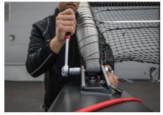
3 Attach the tightening line to the main beam, tension the line in the aft beam and tie off.
