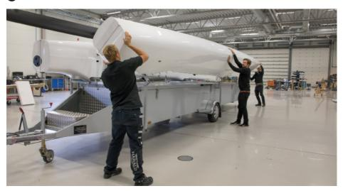
4 Put on the trolleys. They are labeled forward, FWD, and aft, AFT.
