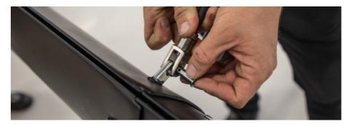
The diamond turnbuckle needs to be properly greased to function. It's a good opportunity to clean and service the turnbuckle when the mast is disassembled. Unscrew and remove the bolt entirely, do not remove the hanger from the mast. Clean the bolt, bronze nut and washer. Put grease on the entire thread of the bolt and bronze nut and on the washer.
