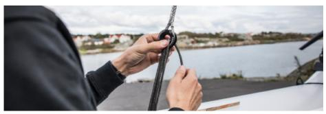
TIP! If it is not possible to tension the front stays due to that the side stay tension is to high, ease the side stays off to be able to tension front stays.
