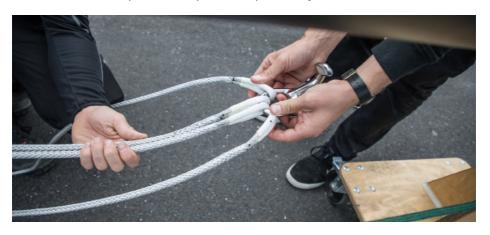
3 Lash the stays with at least 4 laps and tie off so that the load is evenly distributed, as shown in picture. The lashing length is approximately 400 mm measured from the stainless pin to the top of the friction ring on the stays.
