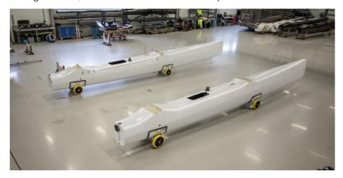
2 Place the main and aft beam in the beam beds.
