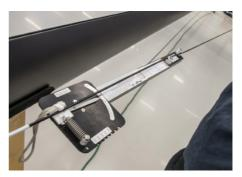
Measure the spreader angle by having a tensioned chock cord rest against the lower diamond and against the respective spreader tip. This measurement should be 190 mm +/- 5 mm. If the spreader angle is NOT as required, take the diamond tension off, adjust the spreader adjustments and repeat procedure until required angle is achieved.
