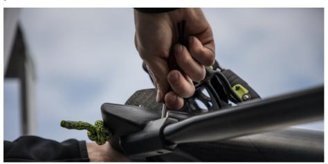
Tighten the strut bolts to 20 Nm using a torque wrench.
