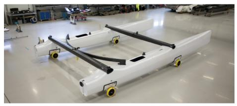
TIP! Make sure to clean the surfaces from grease rests and/or dirt. For any bumps or irregularities that are not coming off, use a 240 grid sandpaper. The surface needs to be even for the best fitting off the beams.
