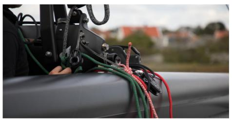
TIP! A small ease of the stepping line will make it easier to get the mast into place.
