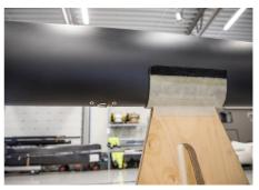
TIP! Have the mast leading edge pointing downwards and use the Cunningham line to tie the mast winch to the stand to keep the mast in this position. The mast will be easier to continue assemble in this position.
