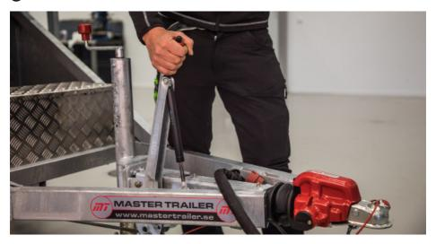
2 Unlock the handles so that the hulls can be folded down.
