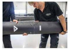
TIP! Have one person at the bottom of the mast, one person holding the bottom section still at the stand closest to the joint and one person at the top of the mast. The person at the joint guides the person at the top to move the top of the mast so it slides on nicely.
