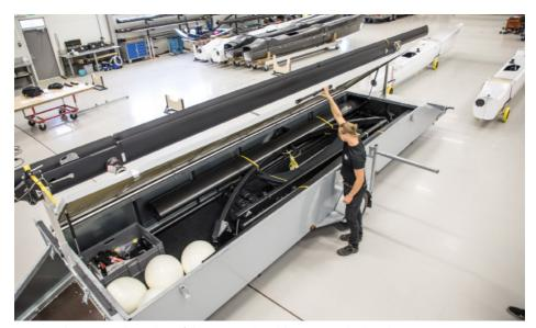
TIP! You do not need to take off the mast to be able to open the hatch.
