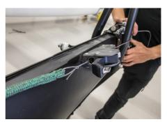
6 Remove the top sheave to insert the main halyard. Use a mouse line to guide the halyard down the luff track. If the halyard is new, connect the main halyard loop by first doing one half hitch with the loop in between and then one half hitch at the end of the halyard.
