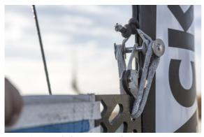
TIP! Lube the luff of the main sail for an easier hoist.
