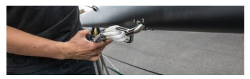
8 Attach the boom to the mast and place it so that it rests on the port hull in front of the main beam.
