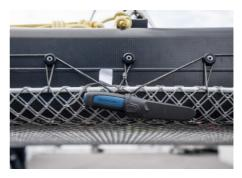
• Attach daggerboard stop line system with the loose ends tied off at the eye bolt on each side and the carabiners in a slider on the opposite side.
