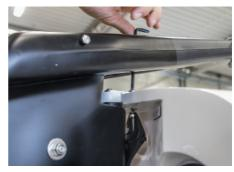
3 Attach the rudder locking arms to the Dyneema locking loops.
