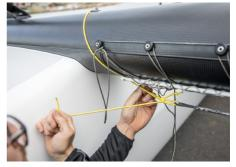
2 Attach tow line around the main beam on the port side of the mast. Make sure the tow line is not tied in around the capsize lines!
