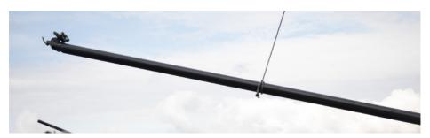
3 Connect the struts to the bowsprit by lowering the bowsprit and guide the struts into it.
