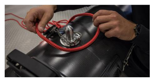
Mount/check override protectors. Remember that with a loose tensioned trampoline the angle of the gennaker sheet going onto the winch will vary.
