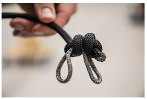
TIP! The halyards need to have a diameter of 8mm to prevent the halyards to come out through the luff track. Do not remove the cover or use lesser diameters.
