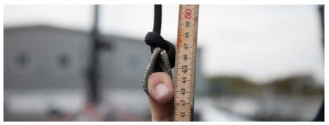
4 Measure the side stay tension using a Spinlock Rig Sense RGS/0508. The tension should be 300 Kg. The black sheave on the gauge should be 1550 mm above the chain plate pin for accurate tuning.
