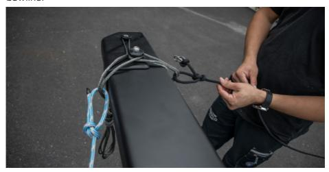
13 Tighten the halyard and tie it off around the gooseneck with a bowline.
