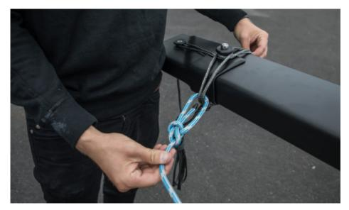
② Attach the main halyard to the upper double boom loop with a bowline.
