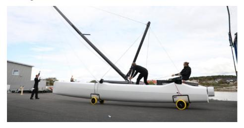
20 Start by lifting the mast foot onto the mast knob.
