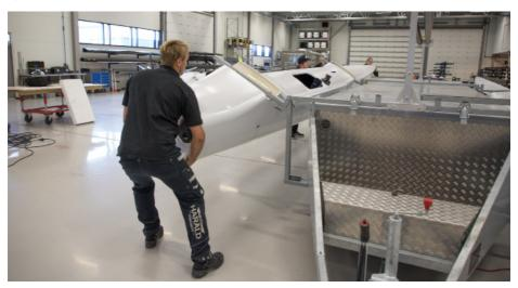
2 Put on the trolleys. They are labeled forward, FWD, and aft, AFT.
