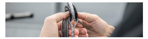
4 If the side stay tension is lower then 300 Kg, tension the side stay lashing using the winch.
