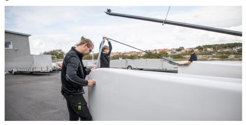
4 Put the strut pins in to lock the struts to the bowsprit and lock the pins with the chock cord.
