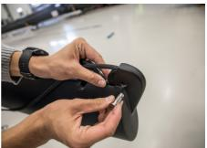
• Connect the main halyard loop by first doing one half hitch with the loop in between and then one half hitch at the end of the halyard.
