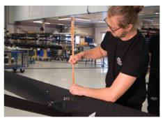
(5) When the spreader angle and the diamond tension are set, tape all pins to avoid any wear or damage to the sail and rig.
