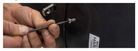
4 Lube the mast track to decrease friction when hoisting the main sail.
