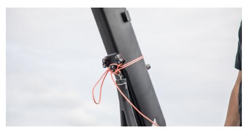
TIP! Have one person at the top of the mast to make sure that it does not fall of the stand when rotating.
