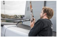
2 Tension the front stays so that the rig ends up centred.
