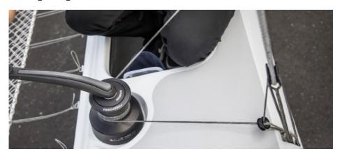
TIP! To prevent damage to deck and lashing, use a soft shackle with friction ring so that the lashing does not run over the deck.
