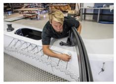
TIP! Easiest way is to be two persons, one from each hull. Be careful so that the glass fibre rods are not scratching the hulls.
