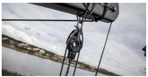
TIP! Use cable ties to make sure that the shackles that connect the two main sheet blocks to the traveler car and double boom loop doesn't come off.
