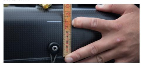
3 Measuring the distance from the measuring mark on the aft beam to the top of the knot. This distance between mark and knot should be 480 mm +/- 5 mm.
