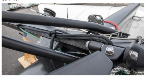
14 If needed, adjust the hoisting line and/or main halyard so that the both lines are tensioned without slack and with the boom in the correct angle, as seen in picture.
