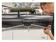
**8** For the aft beam lashing, start with making a loop in the middle of the lashing and then lash outwards from the middle.
