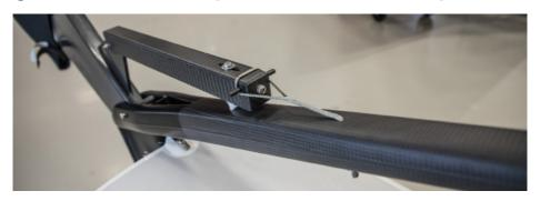
4 Connect the rudders to the the tiller bar using the supplied drop-nose pins.
